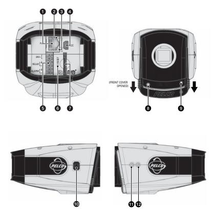
Figure 1. Camera Connections and Features
